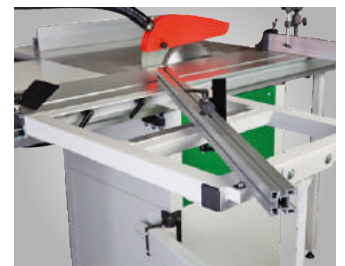
Pivoting telescope stop on sliding carriage
