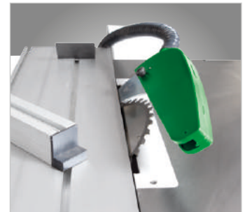
The saw blade pivots through 45°.
