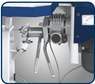
KSO 150 M Sanding unit pivots up to 45° via lever
