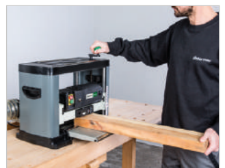
Height adjustment via crank and scale
