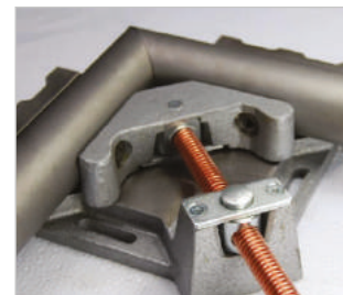
▶ Also suitable for clamping round material
