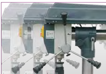
› Variable outreach by displacing the drilling head
