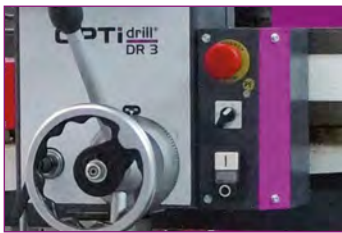
Controls with 24 V DC electrical system
