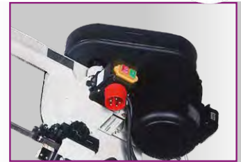
Four speeds Adjustable by shifting the drive belt
