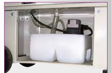
Coolant equipment › Integrated in chassis › Tank capacity 11 litres
