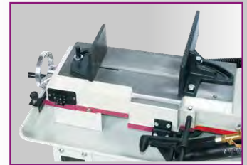
Quick clamping vice › Clamping jaws adjustable from 0° to 45° for mitre cuts
