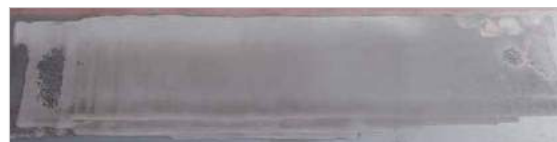
Application grinding stainless steel grinding belt deployed 120 grain for surface structuring
