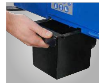
▶ Both swarf catchment containers are easily removable
