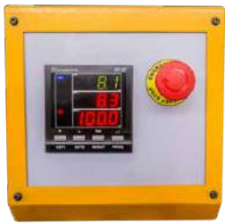
▶ Control panel with digital display and EMERGENCY STOP switch
