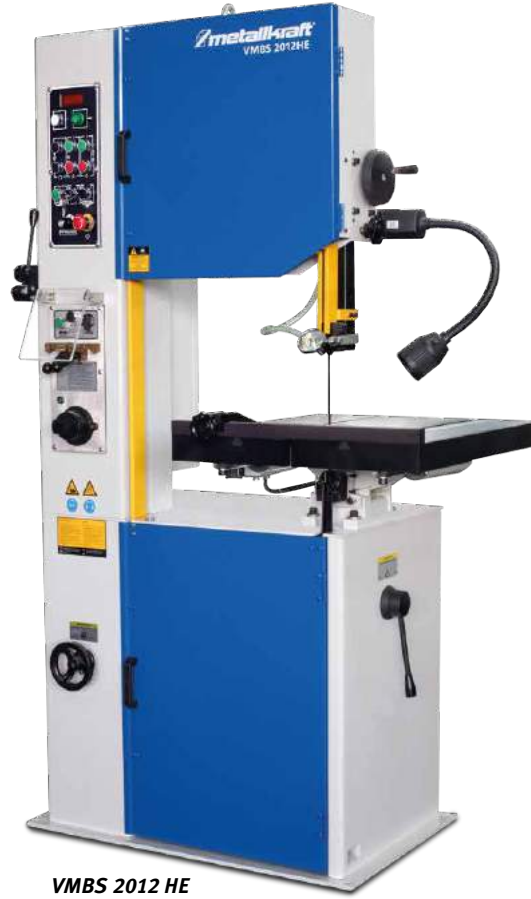
▶ Saw band guide height-adjustable via hand wheel
