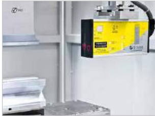
▶ Fiessler AKAS II safety device
