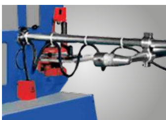
▶ Electrical contact stop (standard as of HPS 55DS)
