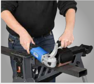
Satin finishing of flat material
