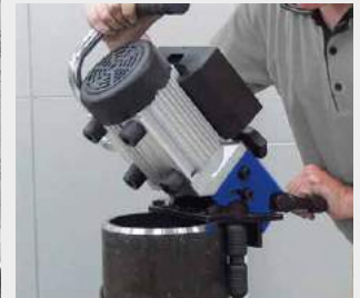
▶ Deburring of pipes possible
