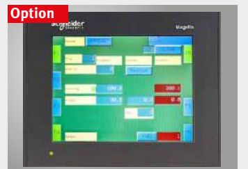
► Optional control Schneider CNC2A , two-axis control for digital angle input and input of the rear stop position with the option of storing bending sequences, motorised rear stop with stop fingers, travel range 15-1 000 mm
