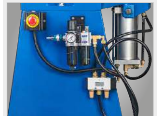
▶ Maintenance unit for pneumatics
