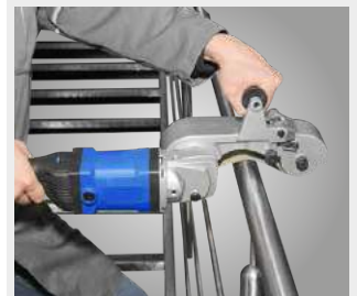
Satin finishing of horizontal round material
