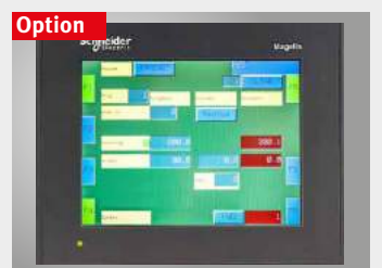
► Optional control Schneider CNC2A , two-axis control for digital angle input and input of the rear stop position with the option of storing bending sequences, motorised rear stop with stop fingers, travel range 15-1 000 mm
