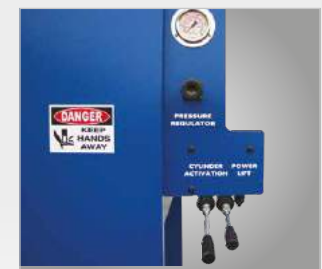
▶ Pressure-sensitive manual lever and pressure gauge
