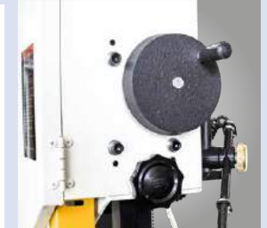
▶ Saw band guide height-adjustable via hand wheel
