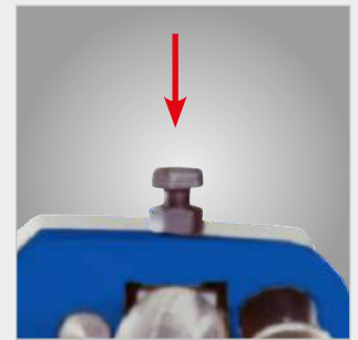
▶ Lubrication via lubricating nipple possible (RBM 305)
