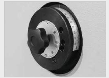
► Standard control MA , manual adjustment of bending angle via ring scale on left side of machine
