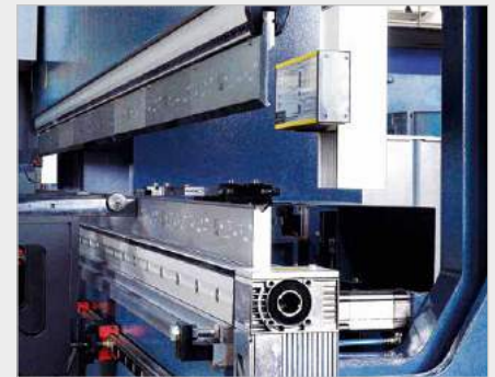
► Hydraulic tool clamping (option)
