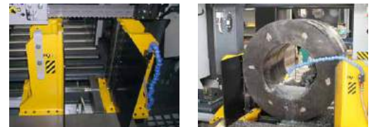
► Clamping of the material upstream and downstream of the cut through two-part vice
