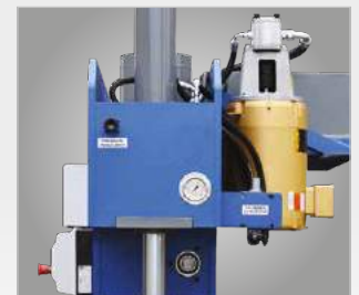
▶ Lateral broaching press with pressure gauge
