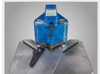
▶ Stops with mitre adjustment
