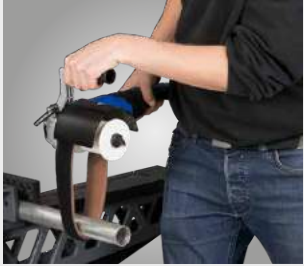
Satin finishing of round steel with Velcro non-woven also for e.g. installed stainless steel railings
