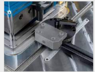
▶ Stops with adjustable blank holders
