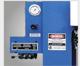
▶ Pressure-sensitive manual lever and pressure gauge
