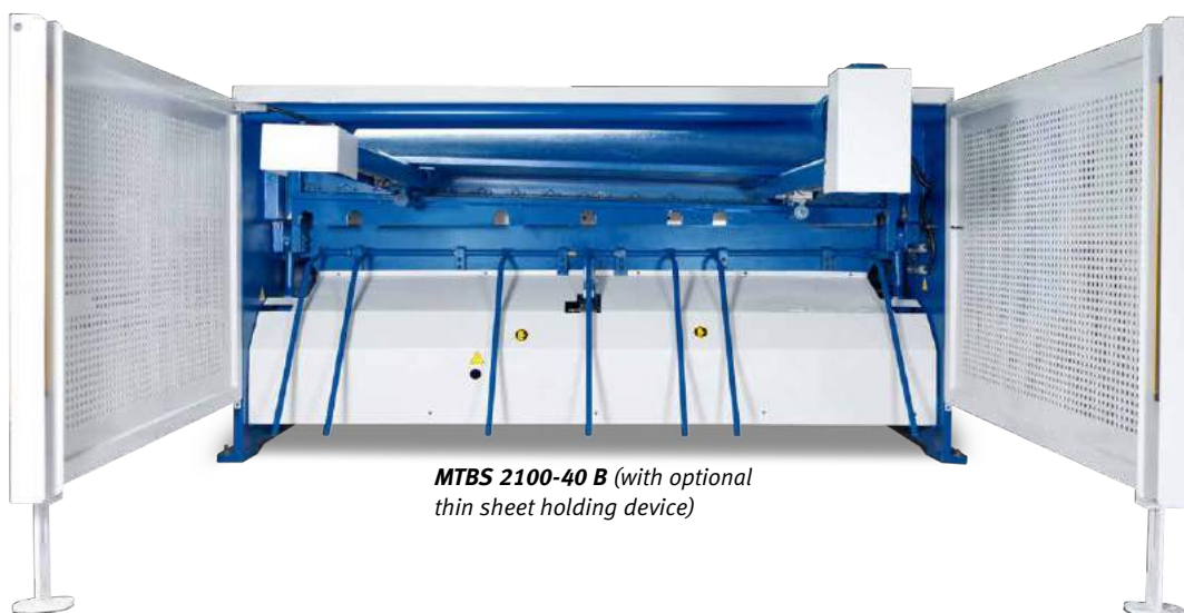
Pneumatic thin sheet support device
