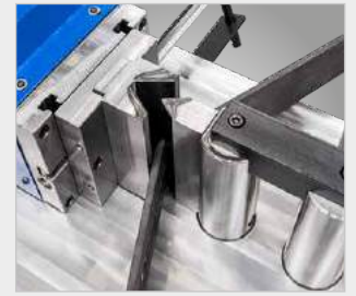
► With quick release mount and side stop with scale
