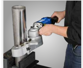
Satin finishing of vertical round material
