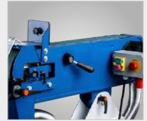
Tension/relieve belt via lever
