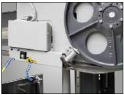
driven cleaning brush for cleaning and maintenance of the saw band
