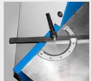
Angle-adjustable side stop with millimetre scale
