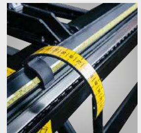
▶ Scale shows bending angles from 0 - 120°
