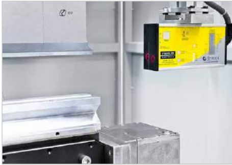
► Finessler AKAS II safety device
