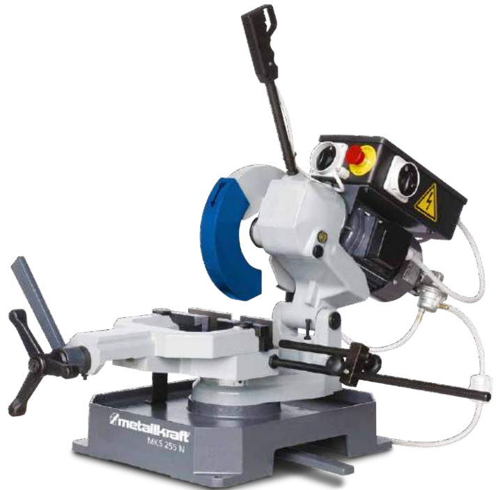
MKS 255 N ▶ Double vice, swivelling from -45° to +45° with quick release
