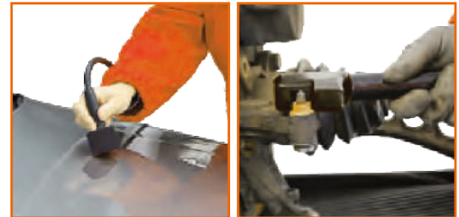
For repairing hail damage without damaging the paintwork
