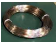
Shiny surface (drawing with liquid lubricant by diamond die)
