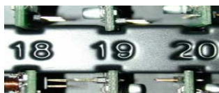
Vacuum formed text for identification of pcb slots
