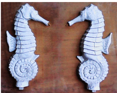
Resin Cast tool of Sea Horse Shape for Cement Casting. 400 x 600 x 50 mm
