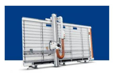
The new Homag Beam Saw makes use of the latest technology allowing us to precision cut large quantities of plywood with optimizing software reducing waste and the new Holzer Wall Saw uses Cam software allowing for greater precision of cut for small works.
